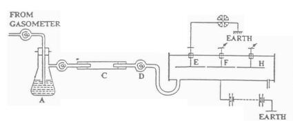
**Figure 4.** Apparatus used by Rutherford and Soddy in 1902<sup>2</sup> to study the emanating power of thorium compounds and to measure the rate of decay of the emanation
